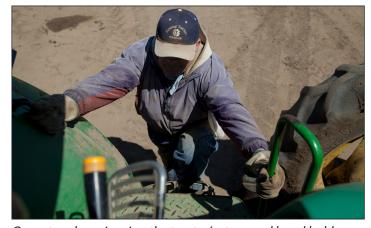
Operator above is using the tractor's steps and hand holds.
